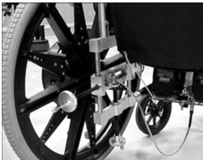
**Figure 2.** Quick-adjust wheelchair axle. Position of axle changed in vertical and horizontal directions with turn of knob.
