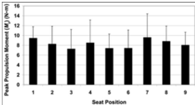
**Figure 9.** Effect of seat position on peak propulsion moment measured at axle.
