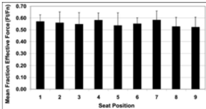
**Figure 8.** Effect of seat position on mean fraction of effective force (FEF) (tangential force/total force). No difference in FEF in change in seat position.
