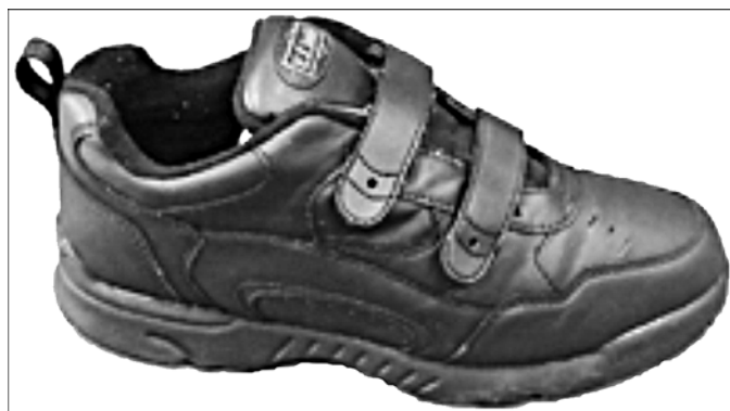
Figure 4. Men’s size 8W, E.Z. Strider ® Walking Shoe (item 75289, Kmart) with synthetic leather upper, synthetic rubber sole, and two Velcro ® straps along dorsal surface used during investigation. Small holes in ends of Velcro straps allowed tensioning by using spring balance.
