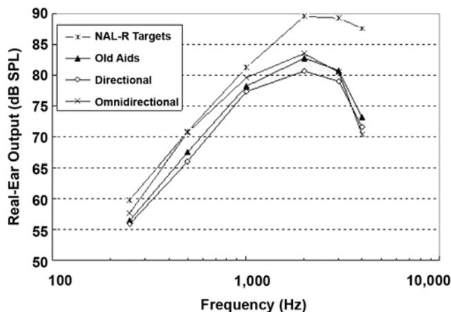
**Figure 7.** Severe group, hearing aid frequency-response characteristics. NAL-R = National Acoustics Laboratory-Revised, SPL = sound pressure level.
