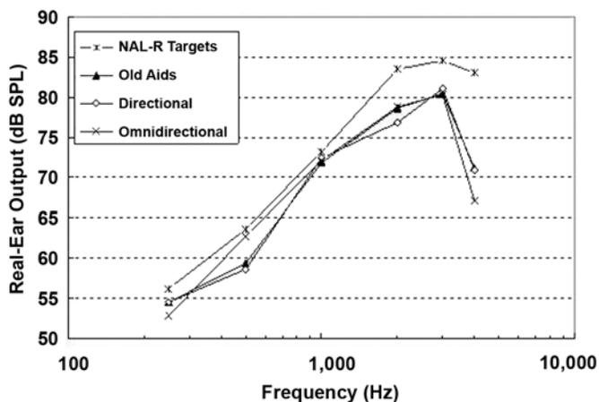
**Figure 6.** Moderate group, hearing aid frequency-response characteristics. NAL-R = National Acoustics Laboratory-Revised, SPL = sound pressure level.
