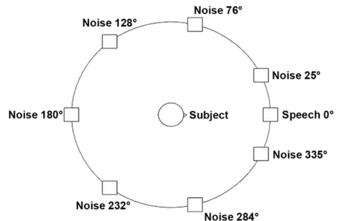
**Figure 4.** Loudspeaker arrangement for Hearing in Noise Test and Connected Speech Test.
