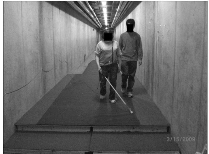
Figure 1. Participant approaching drop-off on 32 ft-long (9.8 m) walkway used in study.
