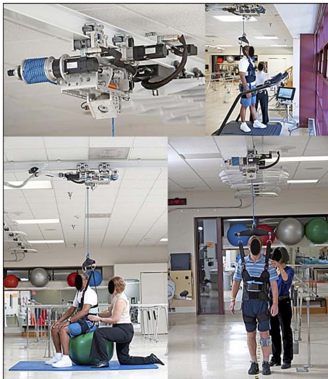
Figure 1. ZeroG gait and balance training system. System is mounted to overhead track that eliminates barriers between therapist and patient. In addition to overground gait and balance training, patients can also practice walking on a treadmill.
