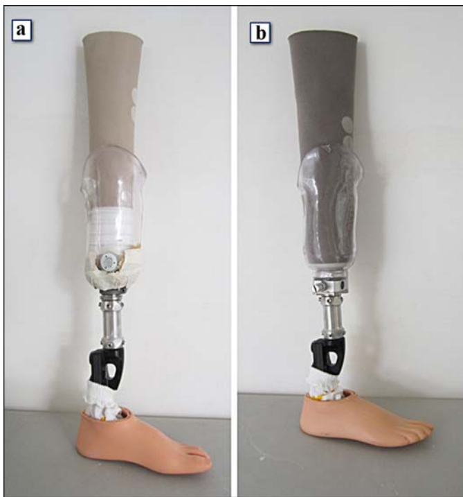
Figure 1. Transtibial suspension systems: (a) Seal-In X5 liner (Össur; Reykjavik, Iceland) with transparent socket and valve and (b) Dermo liner (Össur) with transparent socket and shuttle lock.
