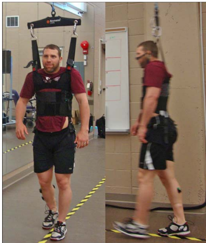
Figure 1. ZeroG overground body weight support (BWS) system. Custom-series elastic actuator travels along overhead trolley providing static and dynamic BWS, allowing individuals to safely practice activities of daily living.
