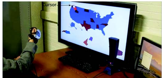
Figure 6. Puzzle game involved grabbing puzzle piece by closing fingers, moving piece by moving hand, and placing piece by opening fingers. Hand and finger movements were detected by P5 Glove (Essential Reality Inc; New York, New York).
