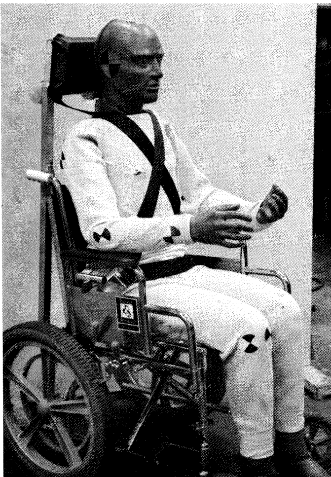
FIGURE 1 Prototype wheelchair add-on restraint system with head restraint.
