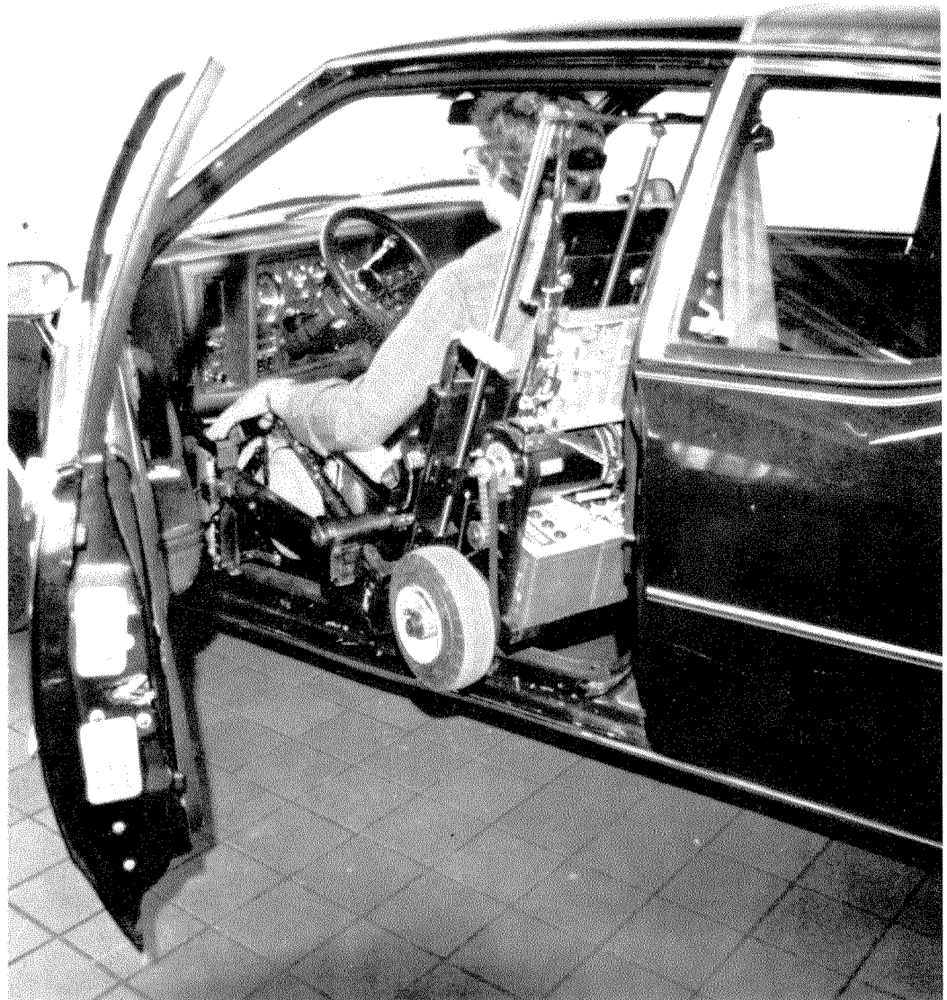
FIGURE 2 Wheelchair is being rotated into driving position by supporting arm.
