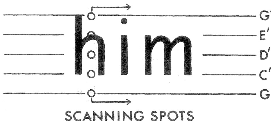
FIGURE 1 Tone generating method of the black-reading Optophone.
